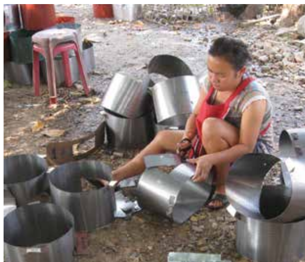
Cutting tin-coated, metal sheet wraparounds for stoves in family-owned business outside Vientiane capital
